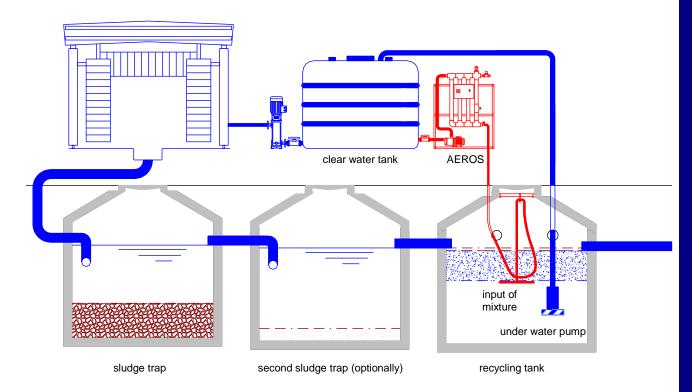
The waste water first flows to the first sludge trap where the most bigger size mud is sedimented.
